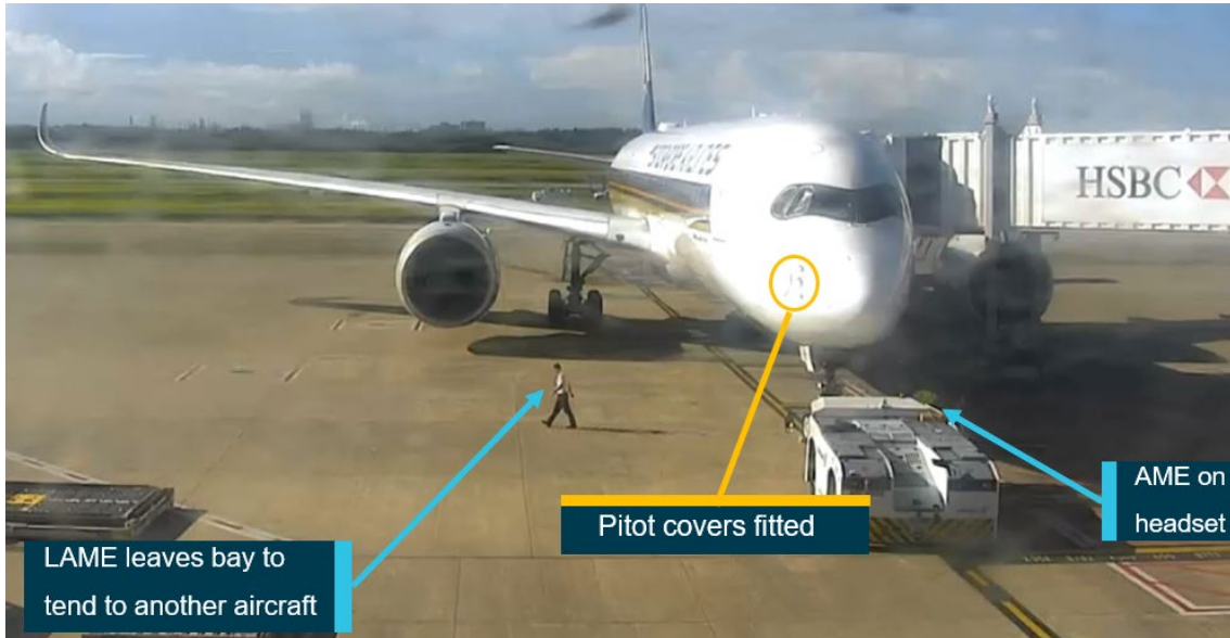
Figure 1: Security footage of bay 81 showing SQ256 4 minutes before pushback with the pitot covers fitted and the LAME moving towards the adjacent bay
