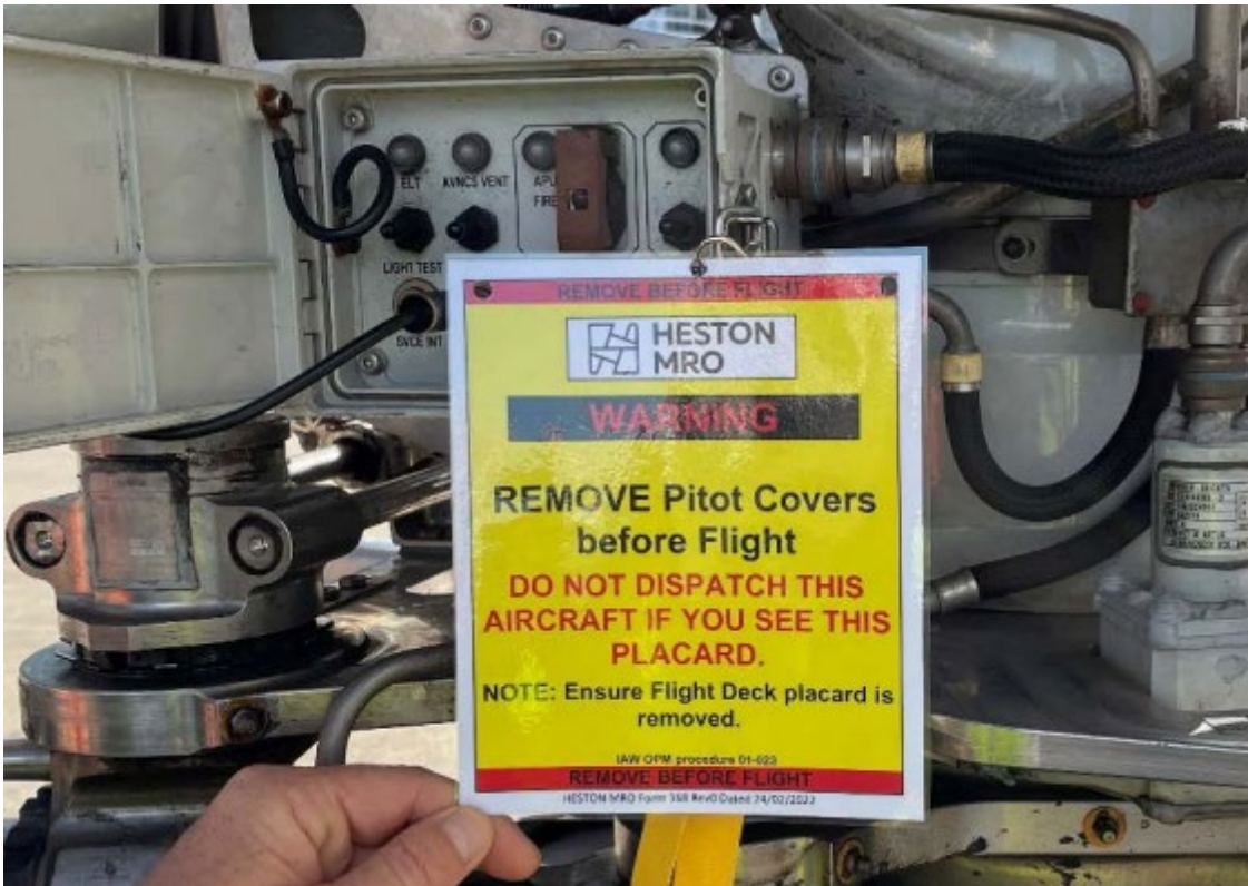
Figure 8: Warning placard fitted to the ground communication panel
