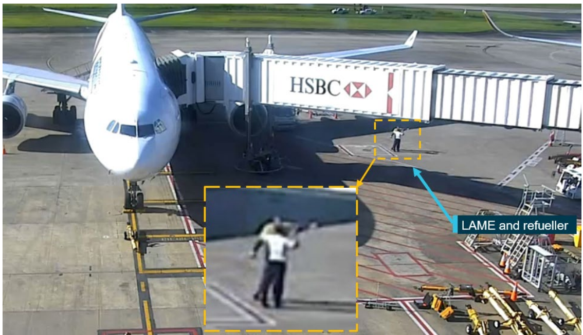
Figure 2: Security footage of the refueller pointing towards SQ256 and informing the LAME that the pitot covers were fitted
