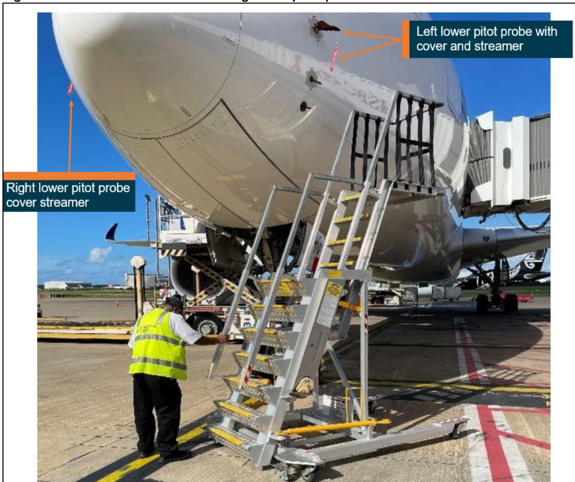
Figure 5: Airbus A350 aircraft showing lower pitot probe covers fitted
