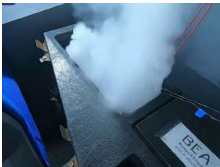
Figure 27: release of smoke during Lithium_Battery_05 test
