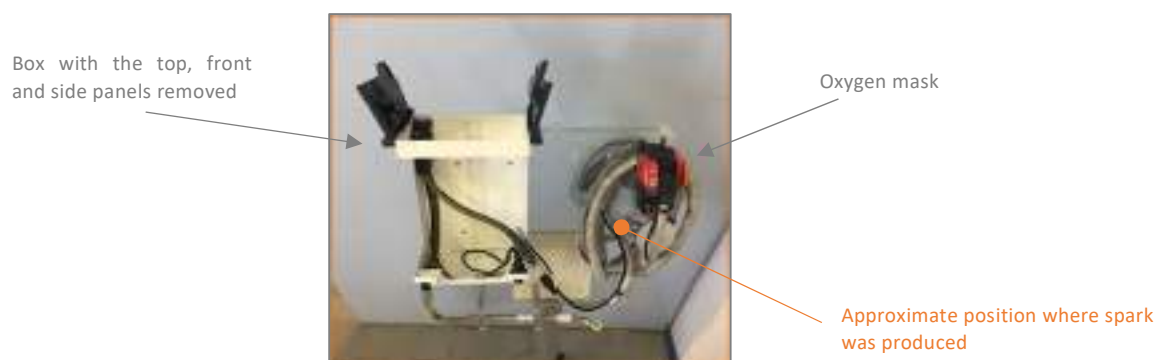
Figure 37: insertion of device in hose of oxygen mask (source: BEA)
