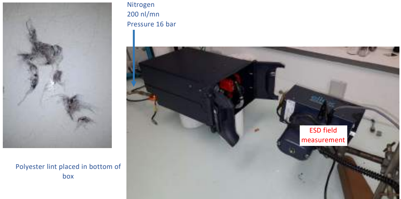
Figure 44: measurement of electrostatic fields created on accumulated synthetic debris at bottom of storage box (source: INERIS)
