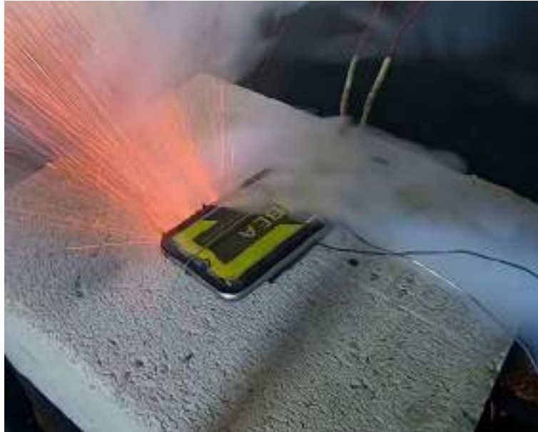
Figure 25: ejection of incandescent particles during thermal runaway of battery (Lithium_Battery_02 test)
