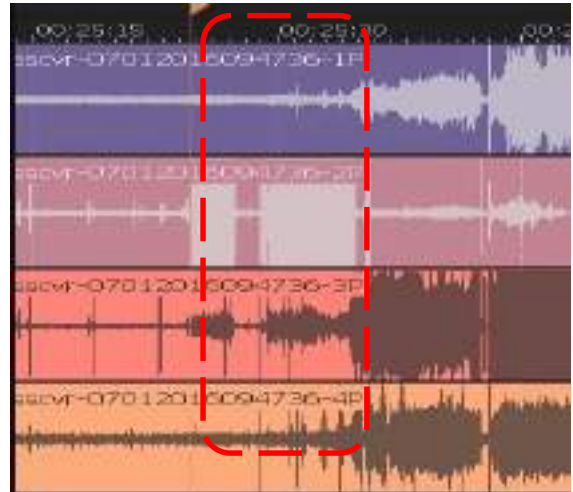
Figure 1.16/9: Wave forms from MSR804 CVR recording
