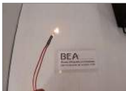
Figure 35: spark production device (source: BEA)
