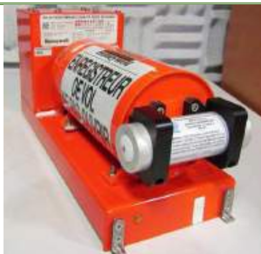
Figure 1.11/8: Example of undamaged Honeywell 980-6022-XXX recorder
