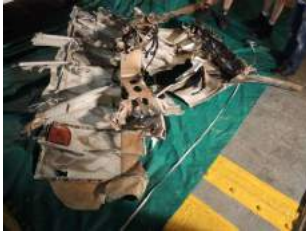
Figure 16: cockpit debris showing black deposits (source: BEA/EEAID)
