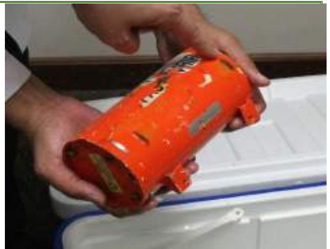
Figure 1.11/5: Two of four mounting brackets missing
