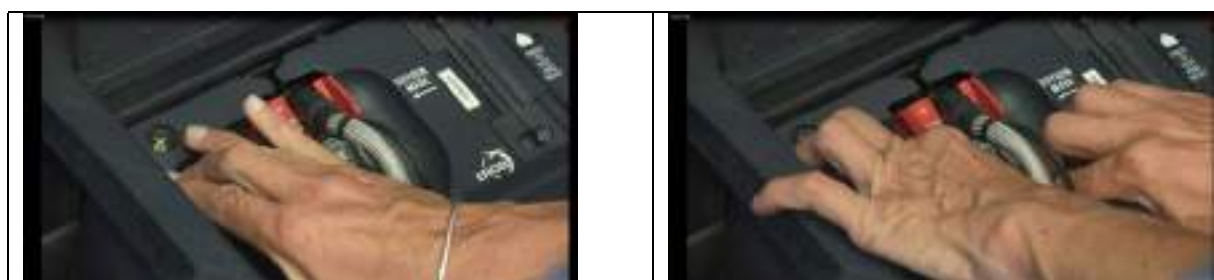
Figure 13: view of actions of oxygen mask test procedure (source: BEA)
