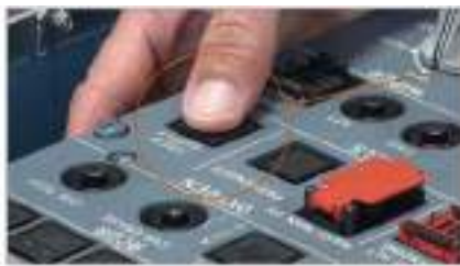
Electrical control of oxygen supply valve
