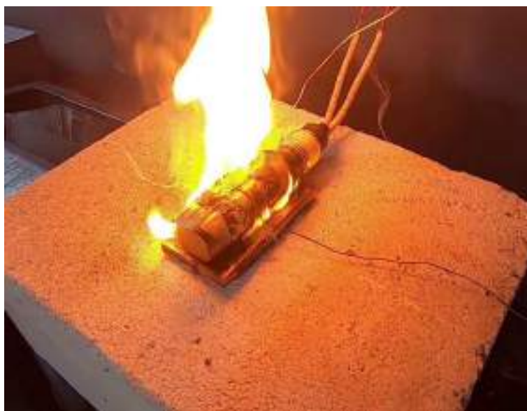
Figure 26: visible flames during Lithium_Battery_07 test
