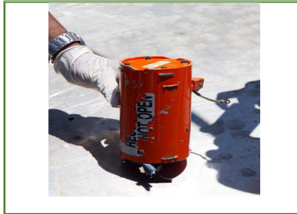
Figure 1.12/4: The CSMU memory unit belonging to one of flight recorders after being recovered.
