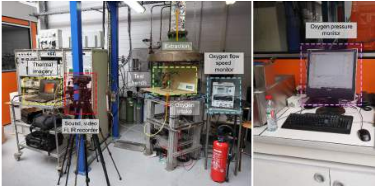
Figure 42: overall view of particle test equipment (source: BEA)
