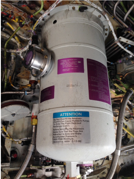
Figure 3. One of the hydraulic reservoirs of a Boeing 737. The warning reads: “Do Not Overfill the Reservoir. Overfill Can Cause Hydraulic Fumes to Enter the Flight Deck and Passenger Cabin.” Notwithstanding the warning, hydraulic fumes can justifiably be said to be an almost permanent component of the interior air of aircraft.
