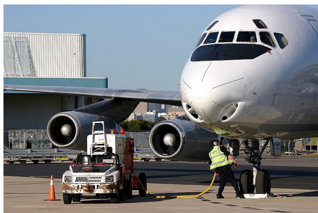
Figure 4. Non-bleed-air technology in 1960. Note the air intakes in the nose of this Douglas DC 8 aircraft. This aircraft used electrical compressors to pressurize and heat the interior.
