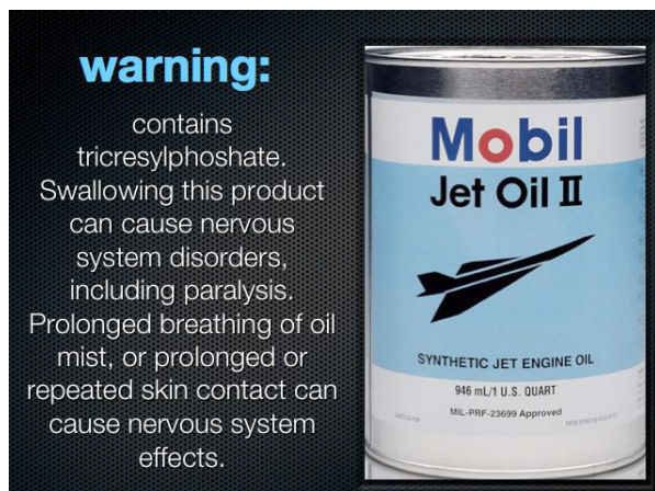
Figure 2. The warning on the back of the can of the most popular engine lubricating oil. Aircrew and passengers are unlikely to ever see this warning.
