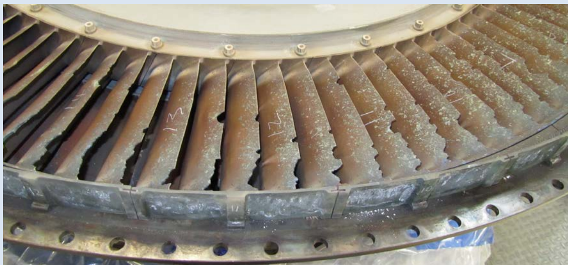
Turbine blades from the damaged Rolls-Royce RB211-524G2-T
