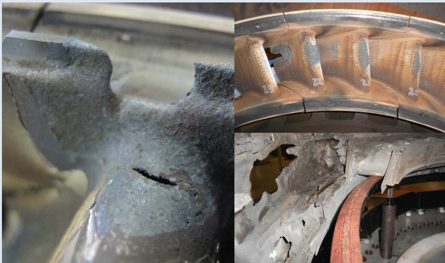
The damaged Engine Alliance 15 GP7200. Clockwise from left; HPT stage-2 nozzle distress, HPT stage-1 nozzles (forward looking aft), Hole in HPT case and missing stage-2 nozzles
