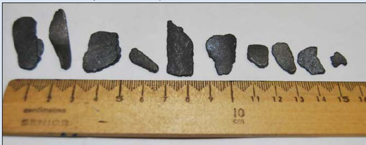
Pieces of engine debris recovered from Riverstone, NSW. Source: NSW Police
