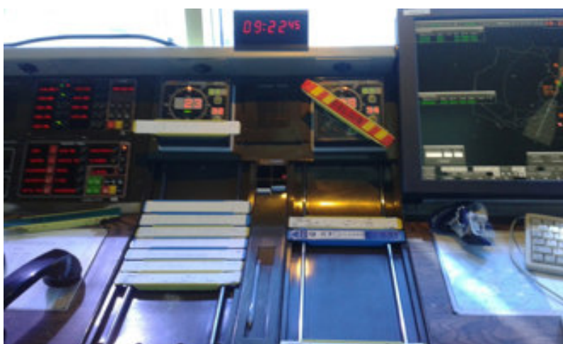
Figure 5. Visual aids at the GCLP LCL post to indicate a runway is closed
