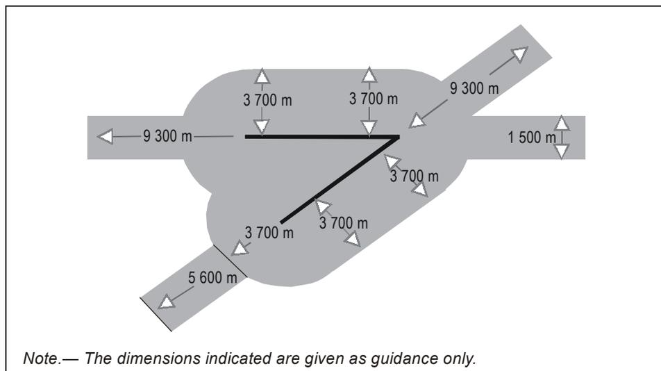
**Figure 5-2. Multiple runway laser-beam free flight zone (LFFZ)**
