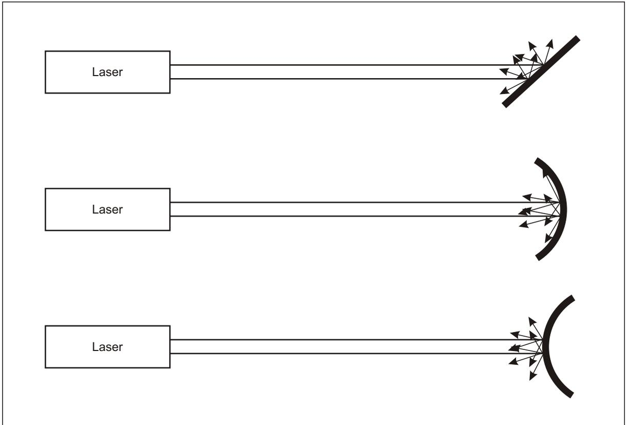
Figure 1-12. Diffuse reflectors
