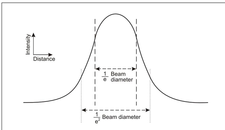
Figure 1-5. Beam diameter
