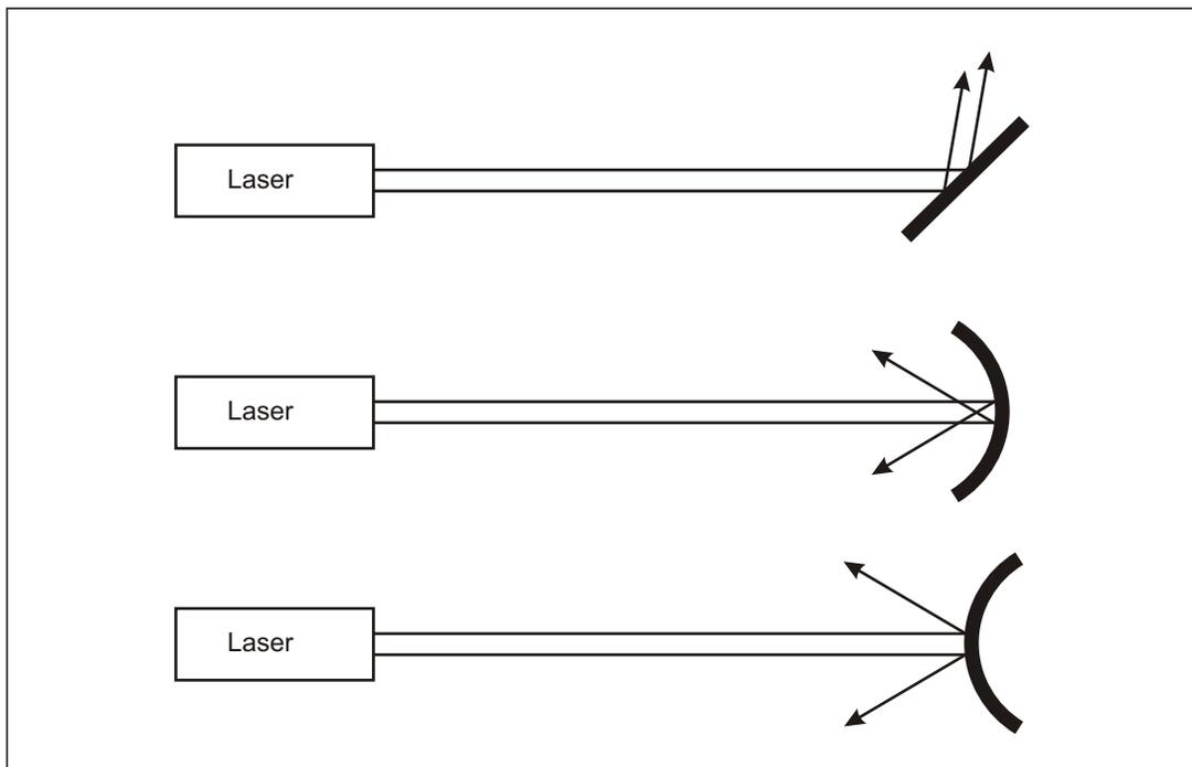
Figure 1-11. Specular reflectors
