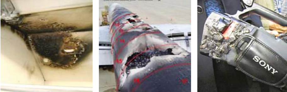
Damage to cabin overhead compartment video camera Hull loss Battery fire
