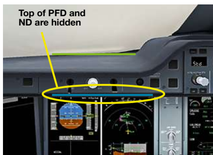
(fig.8) Impaired view on the instrument panel when seated too high
