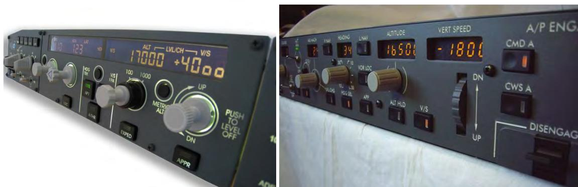
Figure 3: Typical Glareshield Autopilot/Flight Director Interfaces
