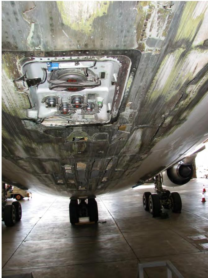
Figure 1: A340 Tailstrike Damage
