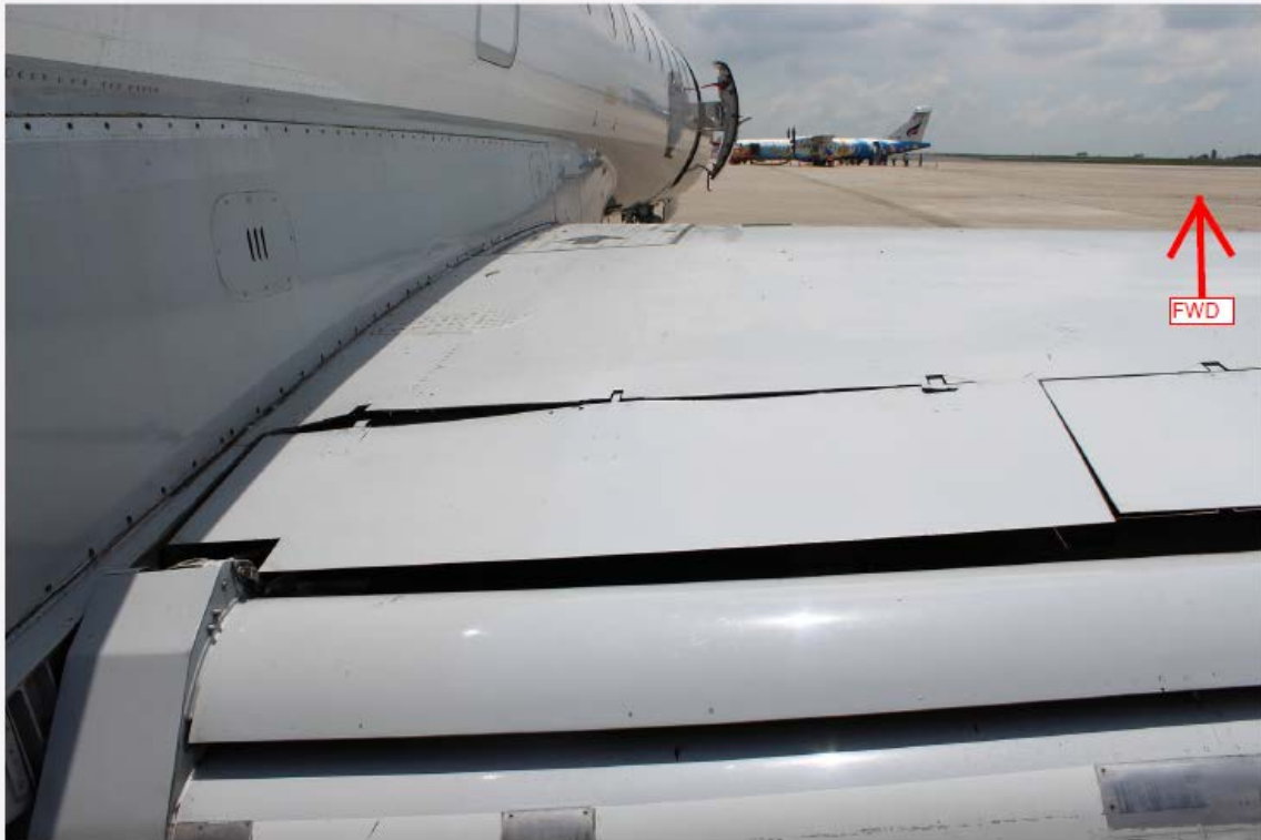
Damages and skin Buckling of RH Inboard Spoiler Panel
