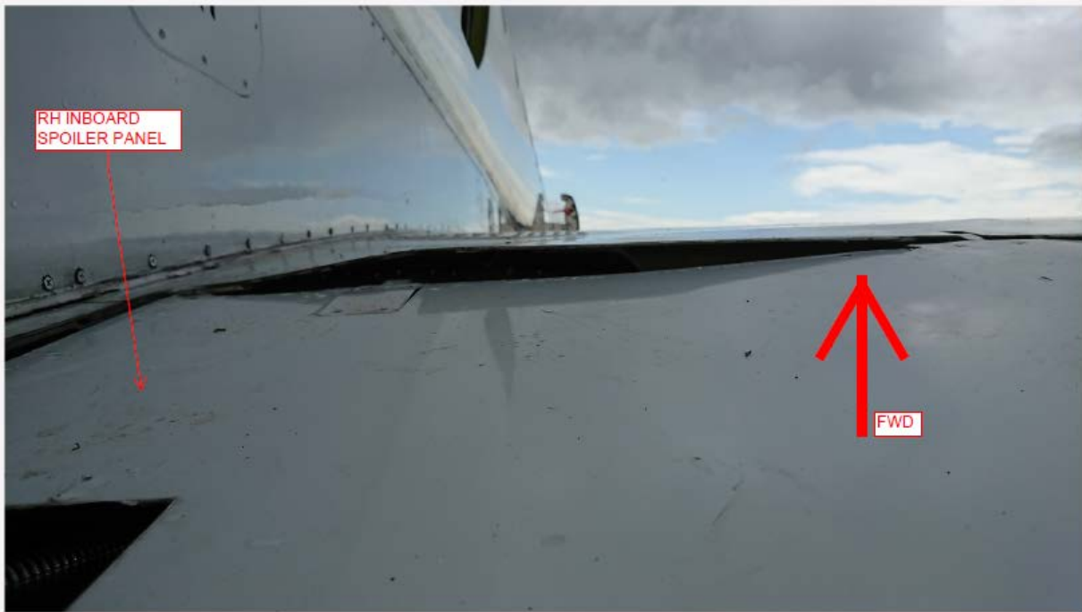
RH Wing, Trailing Edge Skin Buckling ( From Y - 1085.50 + 61 cm )
