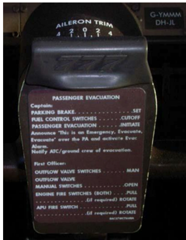
Evacuation checklist on control column
