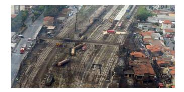
In particular, the **first wagon** *derailed* on plain track. This wagon hit the platform of the train station and overturned to the left, *pulling another four tank cars with it*. These four wagons also derailed and overturned.
