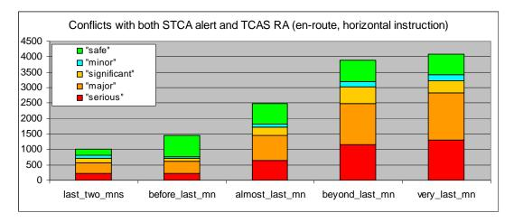
Figure 20: Illustration of STCA performance metric (STCA/ACAS interaction) computed through model-based simulation
