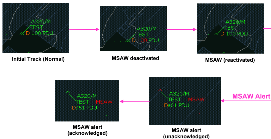
Figure 2-2: Deactivation, reactivation and acknowledgment of MSAW
