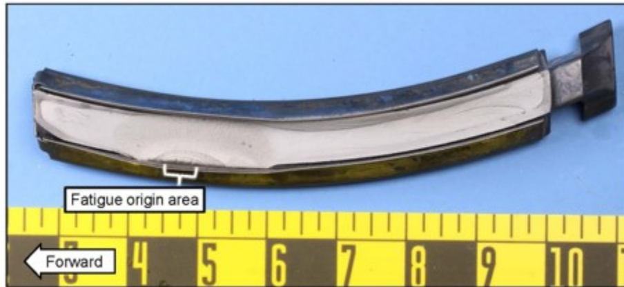
Figure 7. Fan blade No. 23 fracture surface.
