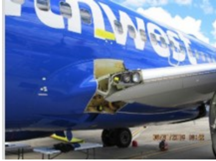
Figure 5. Location of fuselage skin puncture (as indicated by yellow tape).
