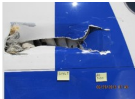
Figure 4. Close-up view of through-puncture on left side of fuselage.
