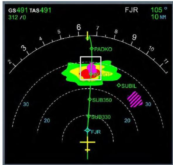
Figure 3. TURB area indication (magenta) on ND [Source: FCOM A380]
