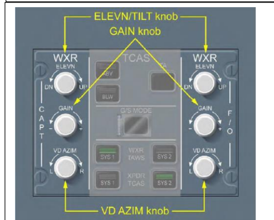
SURV Panel on the cockpit center console
