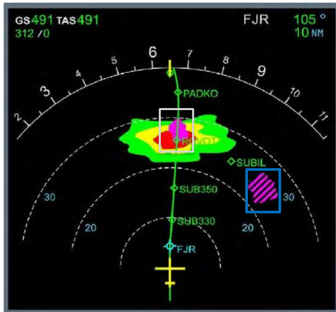
Figure 4. TURB area indication (magenta) on ND [Source: FCOM A380]
