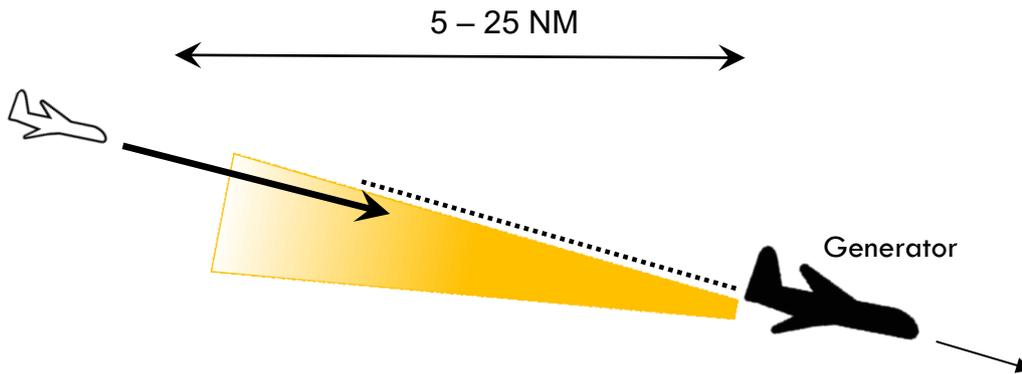
Note: The variability in the generator aeroplane rate of climb or descent makes it quite difficult to estimate exactly, where the vortex is. Consequently, during the en-route phase of flight, pilots should expect possible wake encounters, when other traffics in proximity appear to be on similar tracks ahead, crossing above their level, climbing or descending ahead through their flight path, while wind direction is likely to move the wake towards their trajectory.
