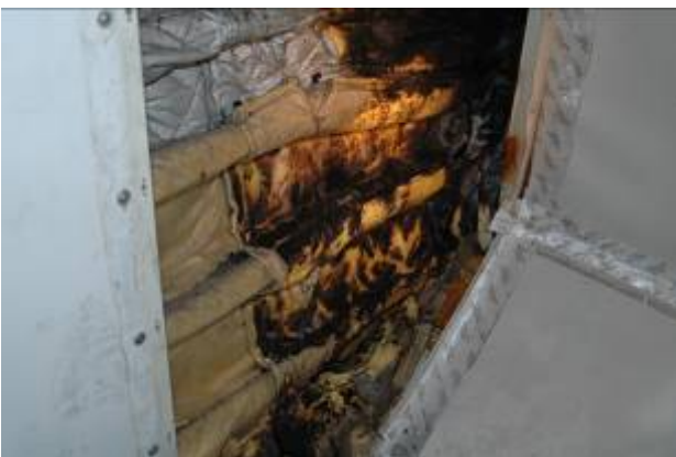
Photos above and below: The charred insulation mats
