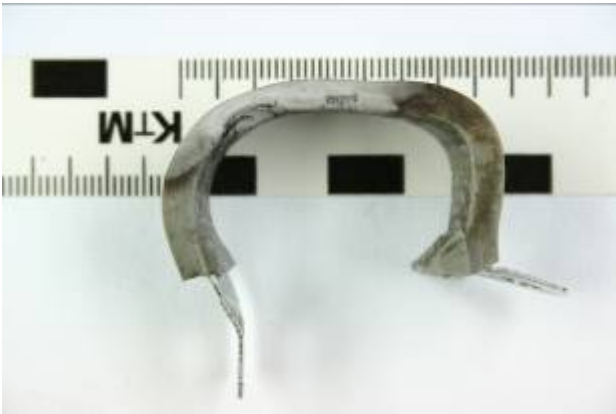
Photos above and below: The defective cable strap
